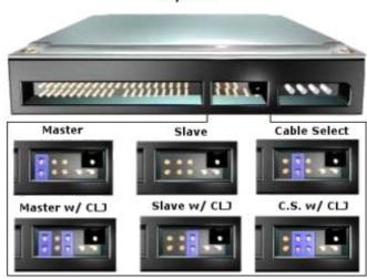
(Master) - A jumper placed over the DS pins configures the drive as a Master.
