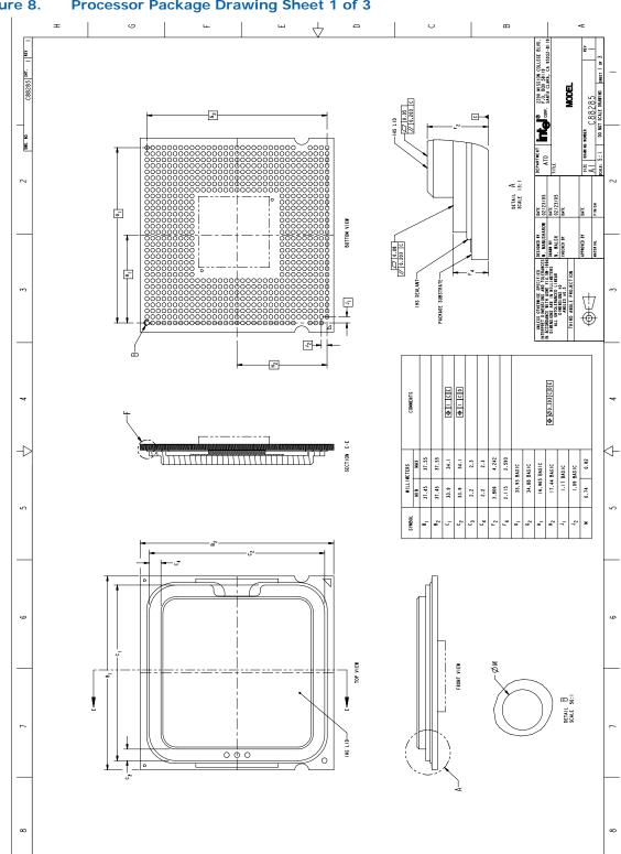
Figure 8. **Processor Package Drawing Sheet 1 of 3**
