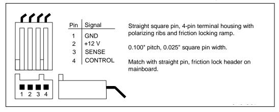
Table 34. **Fan Heatsink Power and Signal Specifications**
