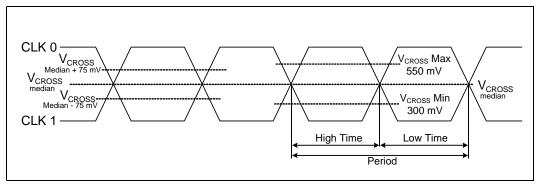
Figure 4. Differential Clock Crosspoint Specification
