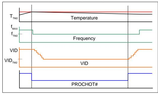
Figure 18. Thermal Monitor 2 Frequency and Voltage Ordering
