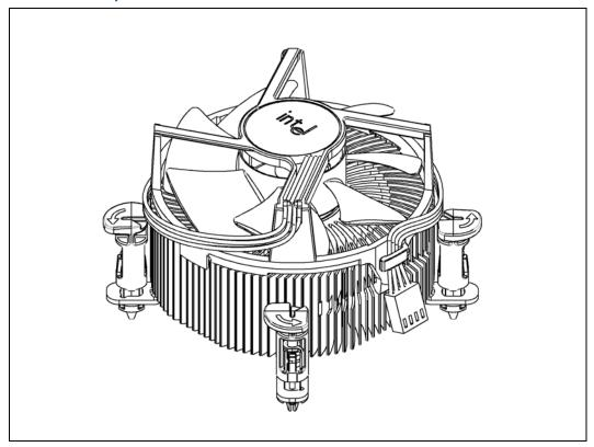
NOTE: The airflow of the fan heatsink is into the center and out of the sides of the fan heatsink.
