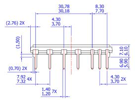
NOTES: UNLESS OTHERWISE SPECIFIED A) THIS PACKAGE DOES NOT COMPLY TO ANY CURRENT PACKAGING STANDARD B) ALL DIMENSIONS ARE IN MILLIMETERS C) DIMENSIONS ARE EXCLUSIVE OF BURRS, MOLD FLASH, AND TIE BAR EXTRUSIONS
