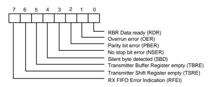
Bit 7: RFEI. In 16450 mode, this bit is always set to a logic 0. In 16550 mode, this bit is set to a logic 1 when there is at least one parity bit error, no stop bit error or silent byte detected in the FIFO. In 16550 mode, this bit is cleared by reading from the USR if there are no remaining errors left in the FIFO.
