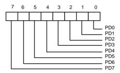
When accesses are made to any EPP data port, the contents of DB0-DB7 are buffered (non-inverting) and output to the ports PD0-PD7 during a write operation. The leading edge of  $\overline{IOW}$  causes an EPP data write cycle to be performed, and the trailing edge of  $\overline{IOW}$  latches the data for the duration of the EPP write cycle.
