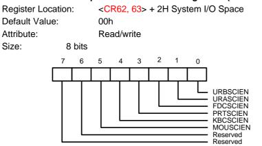
These bits are used to enable the device's IRQ sources into the  $\overline{SCI}$  logic. The  $\overline{SCI}$  logic output for the IRQs is as follows:
