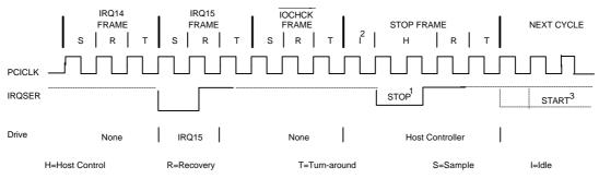
1. Stop pulse is 2 clocks wide for Quiet mode, 3 clocks wide for Continuous mode.
