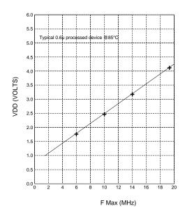
Figure 6-2 F Max vs Vdd
