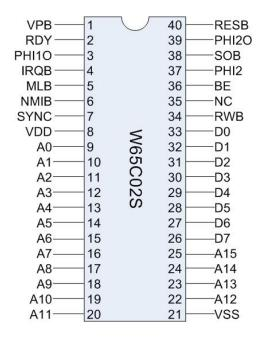
Figure 3-1 W65C02S 40 Pin PDIP Pinout
