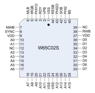
Figure 3-2 W65C02S 44 Pin PLCC Pinout
