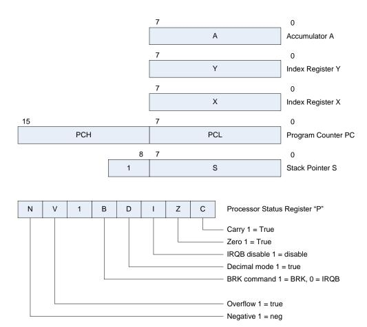
Figure 2-2 W65C02S Microprocessor Programming Model
