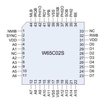
Figure 3-3 W65C02S 44 Pin QFP Pinout
