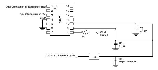
Figure 4. Recommended Circuit Configuration
