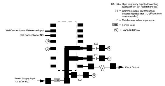
Figure 5. Recommended Board Layout (2-Layer Board)
