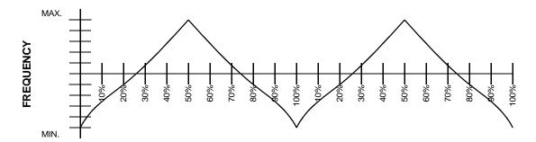
Figure 3. Typical Modulation Profile
