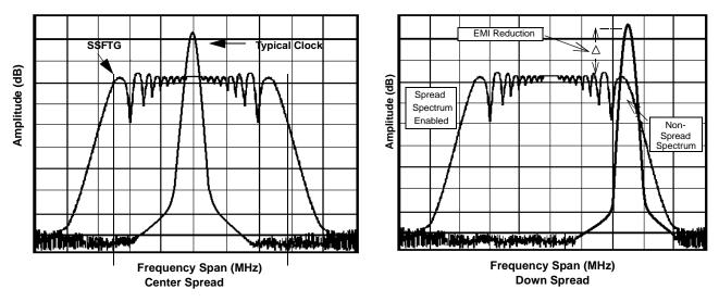
Figure 2. Clock Harmonic with and without SSCG Modulation Frequency Domain Representation
