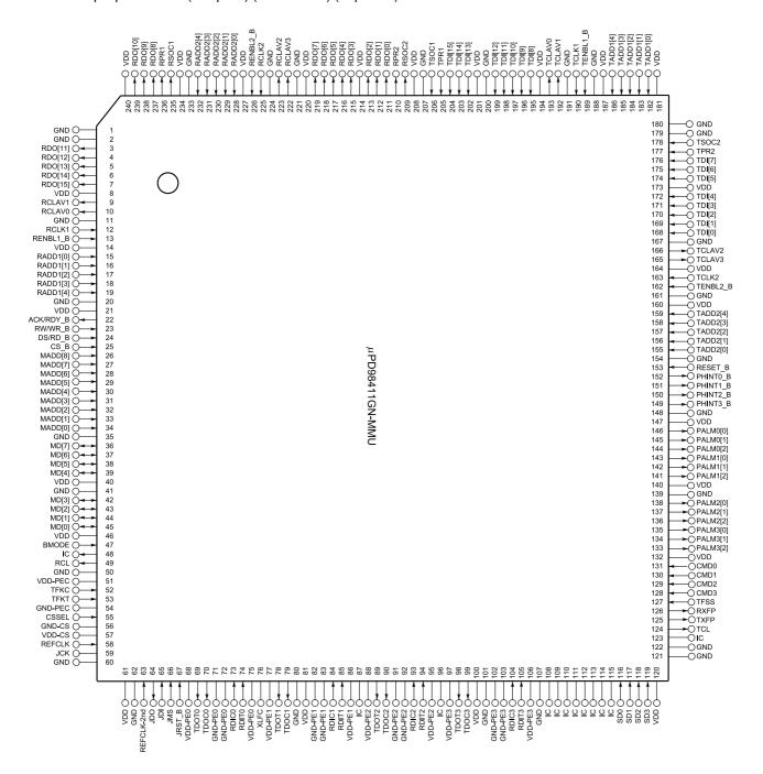
Remark1. IC: internal connect pin. Leave the IC pins open.
