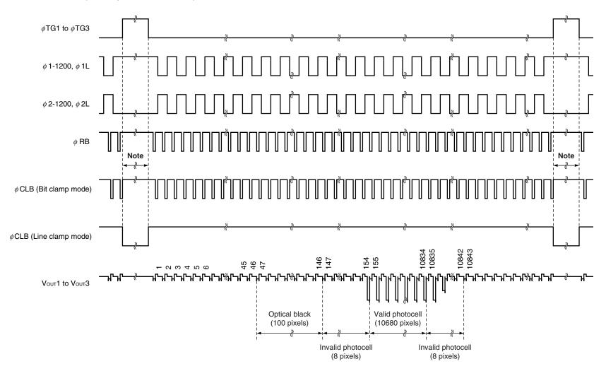
**Note** Set the  $\phi$  RB pulse and  $\phi$  CLB pulse (bit clamp mode) to high level during the  $\phi$  TG1 to  $\phi$  TG3 pulse. And set the  $\phi$  RB pulse to high level while the  $\phi$  CLB pulse is low level at line clamp mode.
