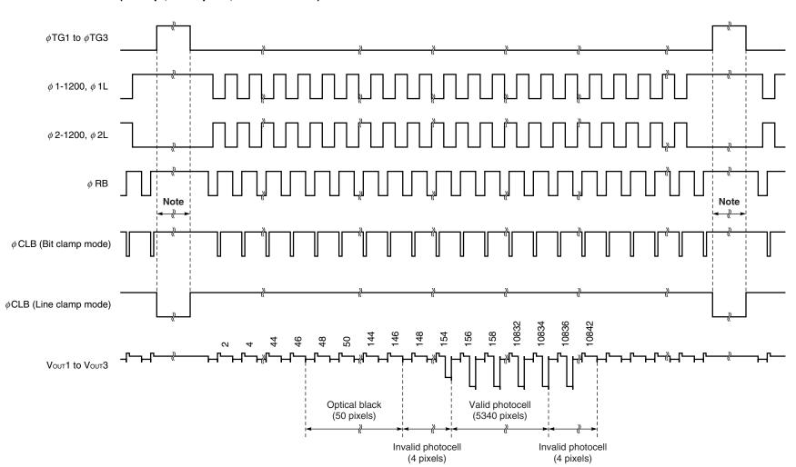
**Note** Set the  $\phi$  RB pulse and  $\phi$  CLB pulse (bit clamp mode) to high level during the  $\phi$  TG1 to  $\phi$  TG3 pulse. And set the  $\phi$  RB pulse to high level while the  $\phi$  CLB pulse is low level at line clamp mode.
