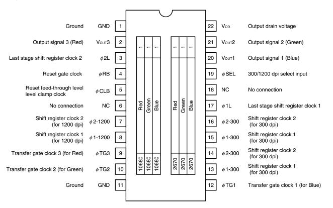
Caution Connect the No connection pins (NC) to GND.
