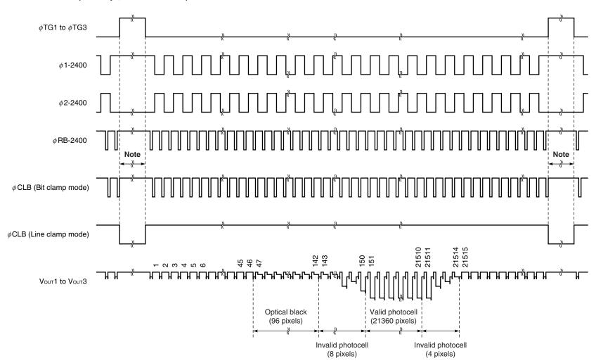
**Note** Set the  $\phi$  RB pulse and  $\phi$  CLB pulse (bit clamp mode) to high level during this period. And set the  $\phi$  RB pulse to high level while the  $\phi$  CLB pulse is low level at line clamp mode.
