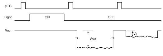
IL (%) =  $\frac{V_1}{V_{OUT}} \times 100$
