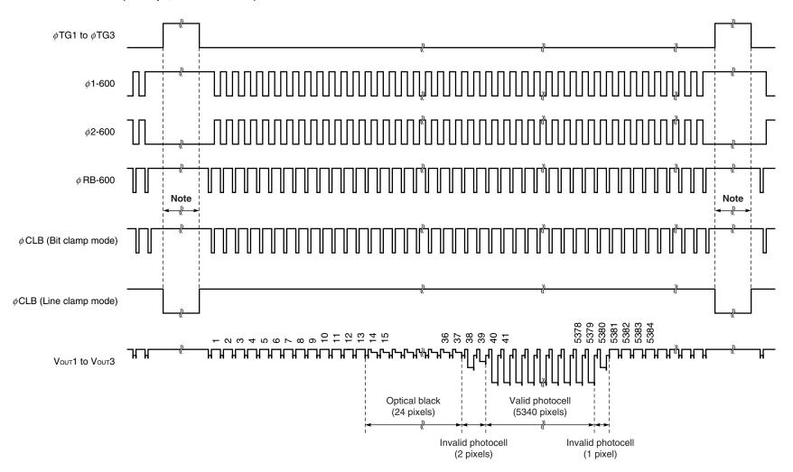
**Note** Set the  $\phi$  RB pulse and  $\phi$  CLB pulse (bit clamp mode) to high level during this period.
