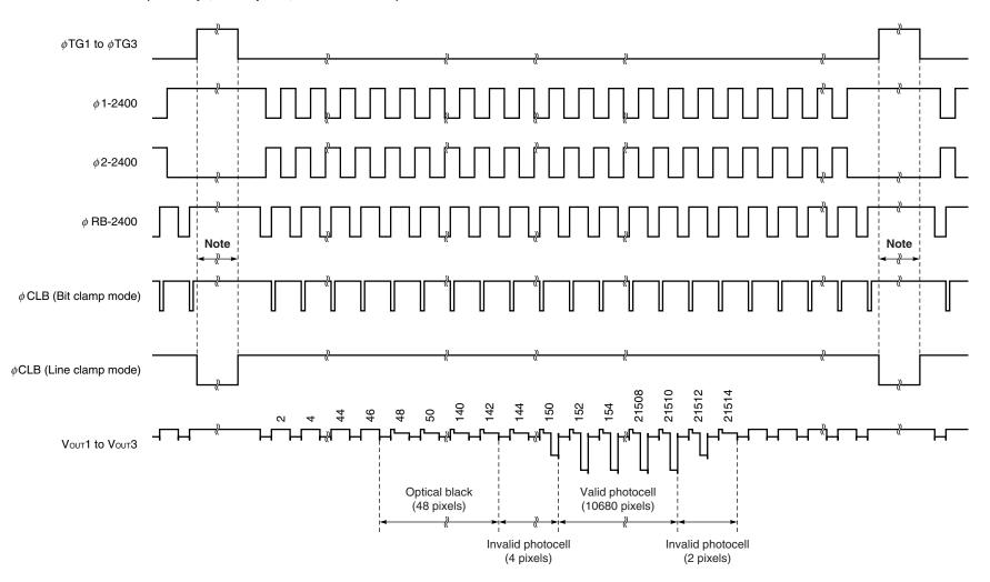
**Note** Set the  $\phi$  RB pulse and  $\phi$  CLB pulse (bit clamp mode) to high level during this period.
