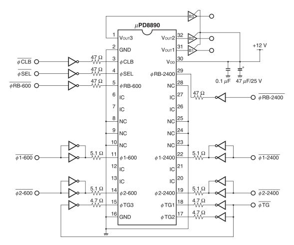
Cautions 1. Leave pins 6, 7, 12, 13, 20, 21, 26, 27 (IC) unconnected. 2. Connect the No connection pins (NC) to GND.
