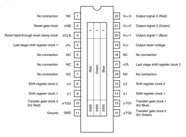
Caution Connect the No connection pins (NC) to GND.
