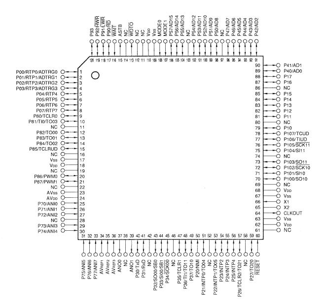
Caution Connect the MODE0 and MODE1 pins directly to the Vss pins.
