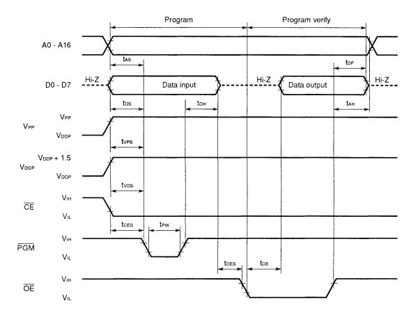
Cautions 1. Vode must be applied before VPP, and must be cut after VPP.
