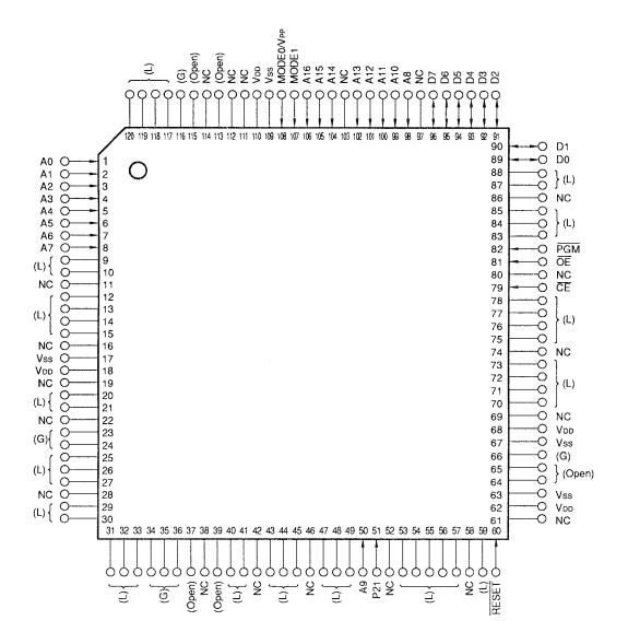
Caution Symbols in parentheses denote how the pins not used in the PROM programming mode should be treated.
