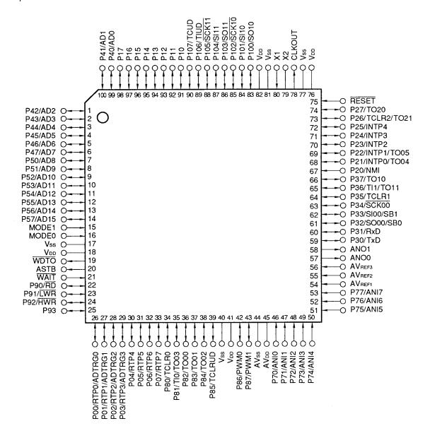
Caution Connect the MODE0 and MODE1 pins directly to the Vss pins.
