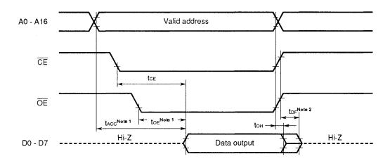
Notes 1. For reading within tacc, the delay of the  $\overline{OE}$  input from falling edge of  $\overline{CE}$  must be within tacc – toe.
