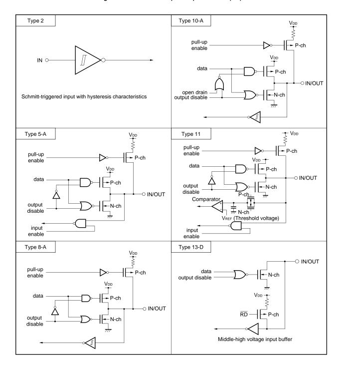
Figure 2-1. List of Pin Input/Output Circuits (1/2)
