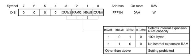
Table 4-1 shows the value settings of IXS to map the internal expansion RAM of the  $\mu$ PD78P048A in the same manner as the respective mask ROM models.
