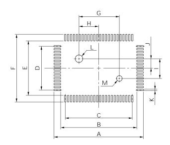
Figure A-2. Recommended Mounting Pattern of V-9200G-80
