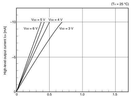
High-level output voltage VDD-VOH [V]
