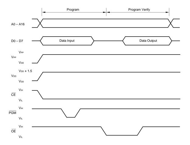
Figure 5-4. Byte Program Mode Timing
