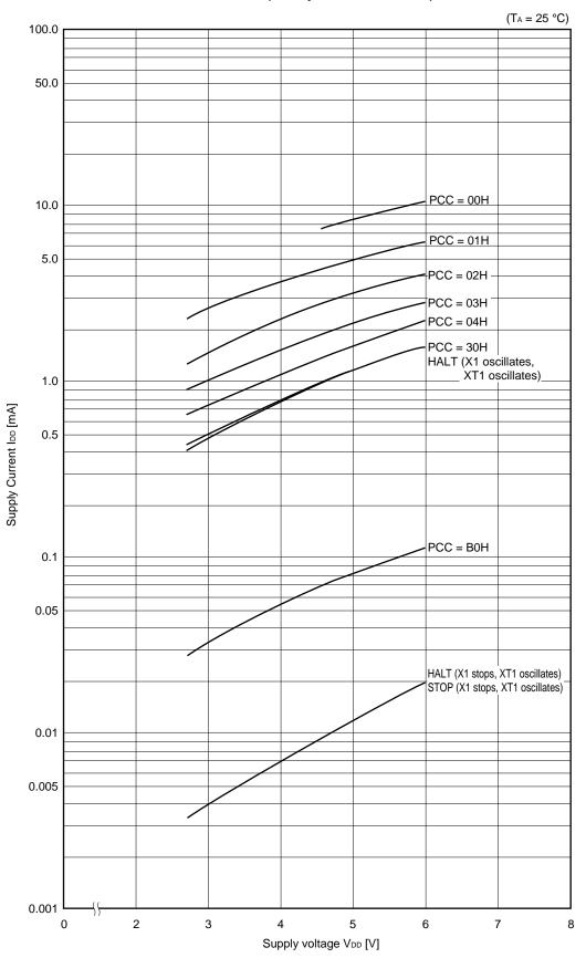
IDD vs. VDD (Main system clock : 5.0 MHz)
