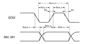
3-wire serial I/O mode with automatic transmit/receive function:
