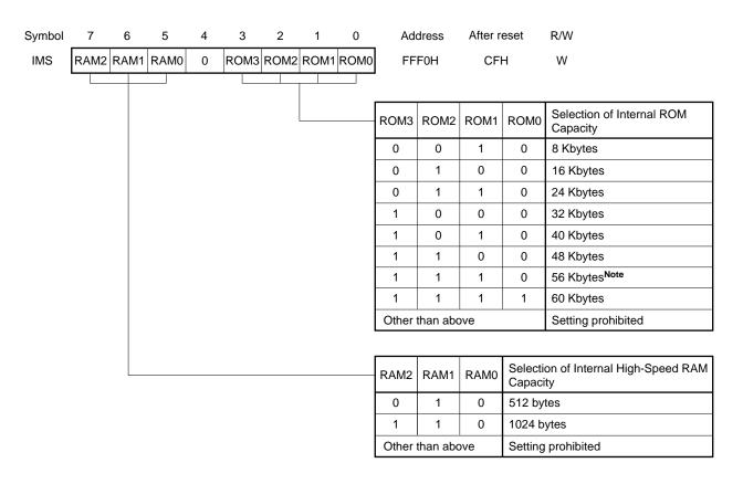
**Note** When the external device expansion function is used, the internal ROM capacity should be set to 56 Kbytes or less.
