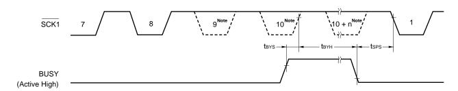
Note The signal is not actually driven low here; it is shown as such to indicate the timing.
