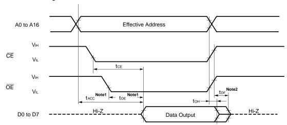
Notes 1. When reading within the tacc range, the  $\overline{OE}$  input delay time from the  $\overline{CE}$  fall time must be maximum of tacc – toe.
