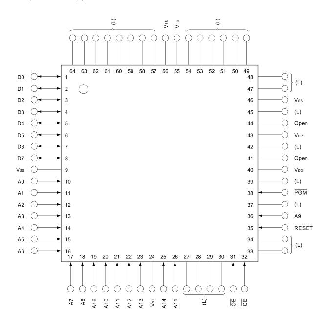
Cautions 1. (L): Independently connect to Vss via a pull-down resistor.
