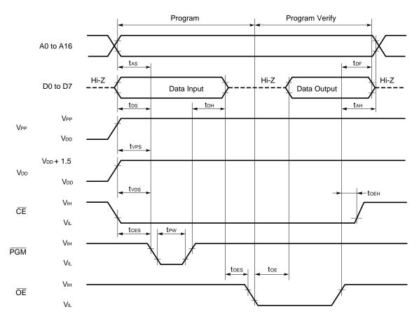
Cautions 1. VDD must be applied before VPP and cut off after VPP.
