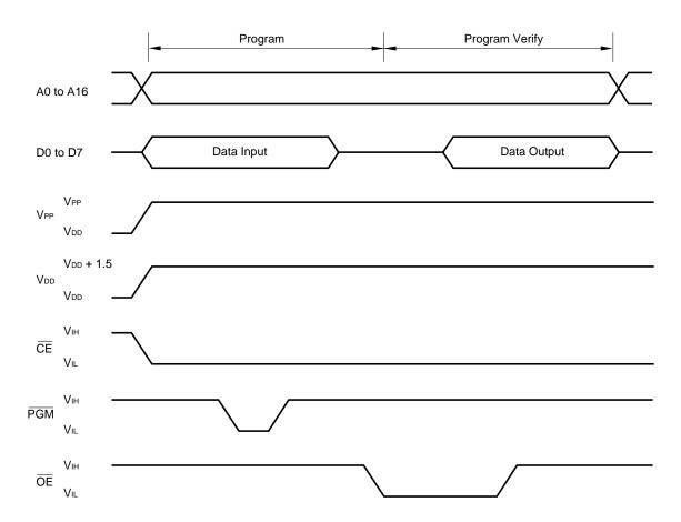
Figure 5-4. Byte Program Mode Timing
