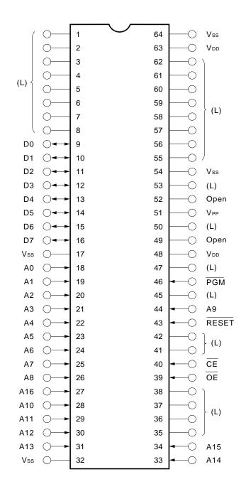
Cautions 1. (L): Independently connect to Vss via a pull-down resistor.
