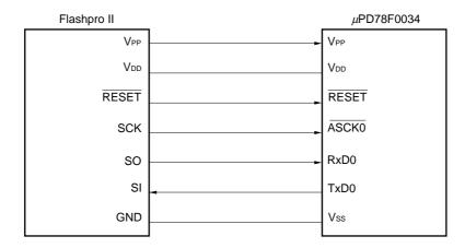
Figure 4-4. Connection of Flashpro II Using Pseudo 3-Wire Serial I/O Method
