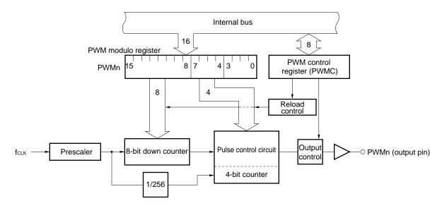
Figure 7-6. Block Diagram of PWM Output Unit
