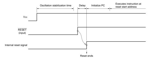
Figure 11-2. Power-ON Reset Operation
