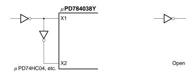
Caution When using the clock oscillation circuit, wire the dotted portion in the above figure as follows to avoid adverse influences of wiring capacitance.
