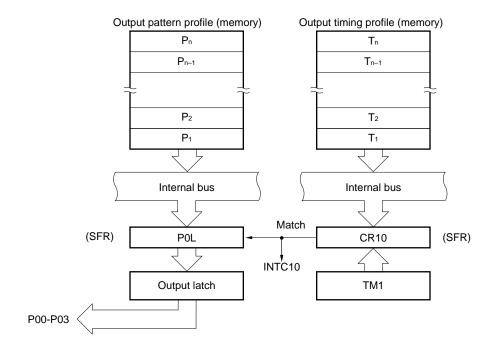
Each time macro service request (INTC10) is generated, the pattern and timing are transferred to the buffer register (P0L) and compare register (CR10), respectively. When the contents of the timer register 1 (TM1) coincide with those of CR10, INTC10 is generated again, and the contents of P0L are transferred to the output latch. When Tn (last byte) has transferred to CR10, vectored interrupt request (INTC10) is generated.
