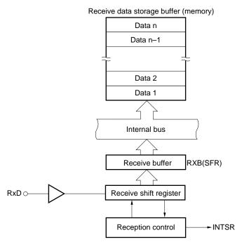
Each time macro service request (INTSR) is generated, the receive data is transferred from RXB to memory. When data n (last byte) has been transferred to memory (when the receive data storage buffer has become full), vectored interrupt request (INTSR) is generated.
