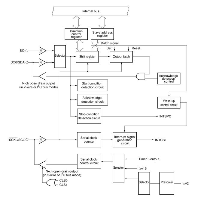
Figure 7-12. Block Diagram of Clocked Serial Interface
