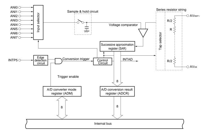
Figure 7-7. Block Diagram of A/D Converter
