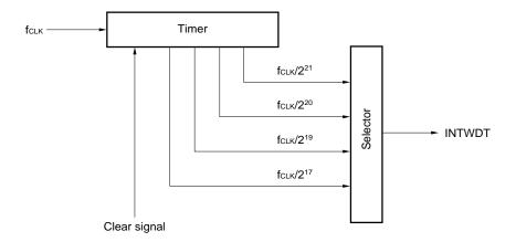
Figure 7-14. Block Diagram of Watchdog Timer
