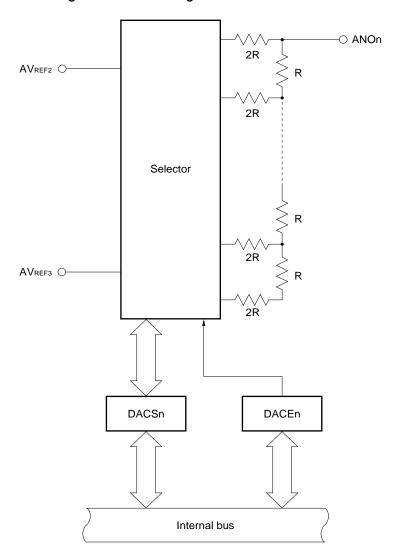
Figure 7-8. Block Diagram of D/A Converter
