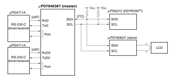
(b) UART + 3-wire serial I/O + 2-wire serial I/O
