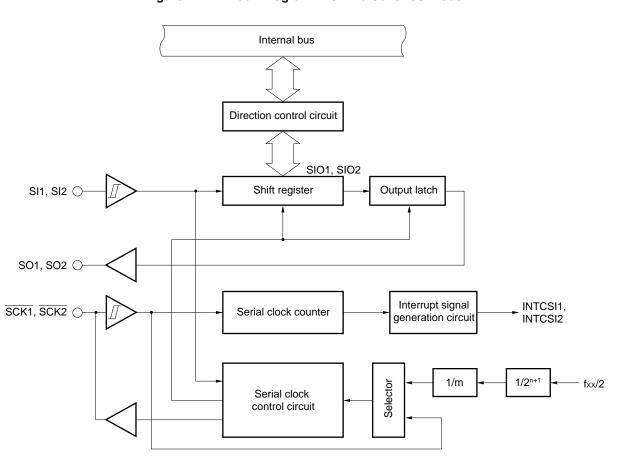
Figure 7-11. Block Diagram in 3-wire Serial I/O Mode
