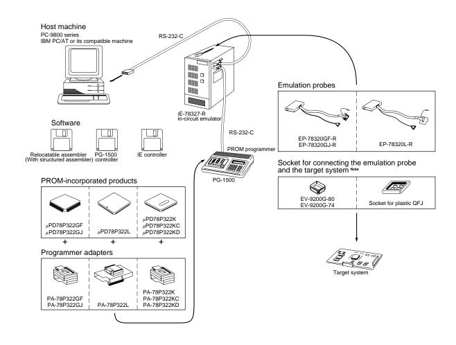
**Note** The socket is supplied with the emulation probe.
