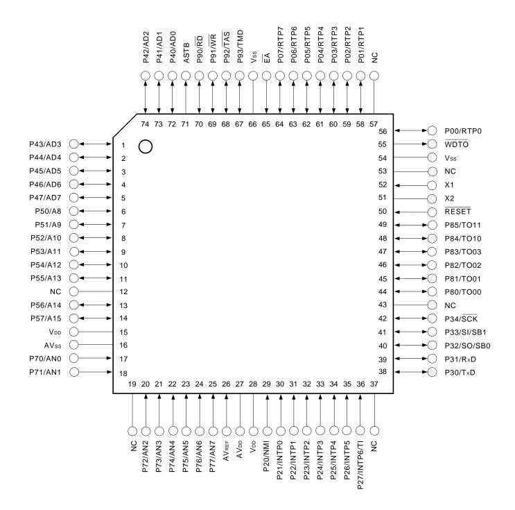
Caution The NC pin should be connected to Vss for noise control (can also be left open).
