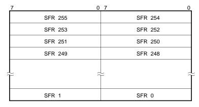
Remark The CCWs of the control registers are mapped in the special function register (SFR) area.
