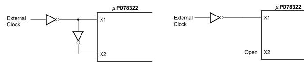
Cautions 1. When the system clock oscillator is used, the following points should be noted concerning wiring within broken lines shown in Figure 3-2, in order to prevent the effects of wiring capacitance, etc.
