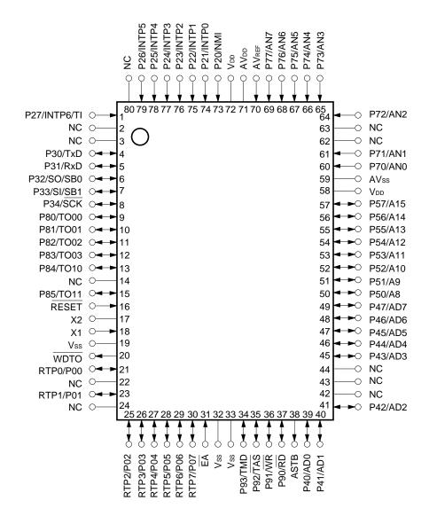
Caution The NC pin should be connected to Vss for noise control (can also be left open).
