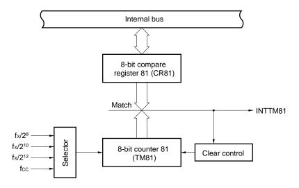
Figure 5-6. Block Diagram of Watchdog Timer
