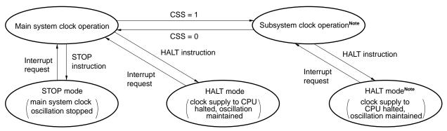
**Note** The current consumption can be reduced by stopping the main system clock.
