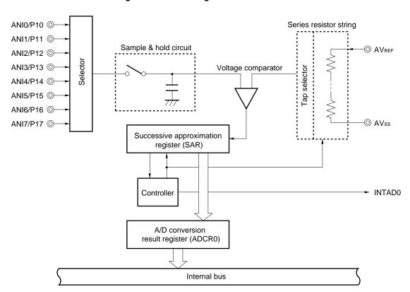
Figure 5-7. Block Diagram of A/D Converter
