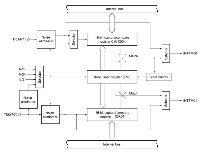
Figure 5-2. Block Diagram of 16-Bit Timer/Event Counter 0 (TM0)
