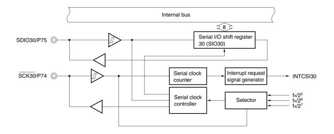
Figure 5-11. Block Diagram of Serial Interface SIO30
