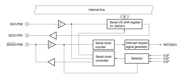
Figure 5-12. Block Diagram of Serial Interface SIO31
