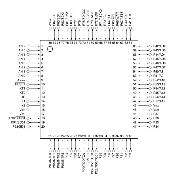
Cautions 1. Connect the IC (internally connected) pin directly to V<sub>SS0</sub> or V<sub>SS1</sub>. 2. Connect the AVss pin to V<sub>SS0</sub>.
