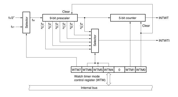
Figure 5-5. Block Diagram of Watch Timer
