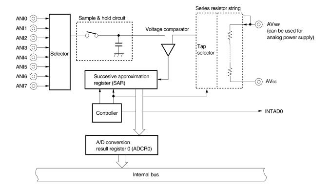
Figure 5-8. Block Diagram of A/D Converter
