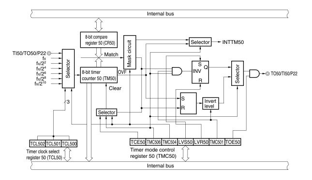
Figure 5-3. Block Diagram of 8-bit Timer/Event Counter 50
