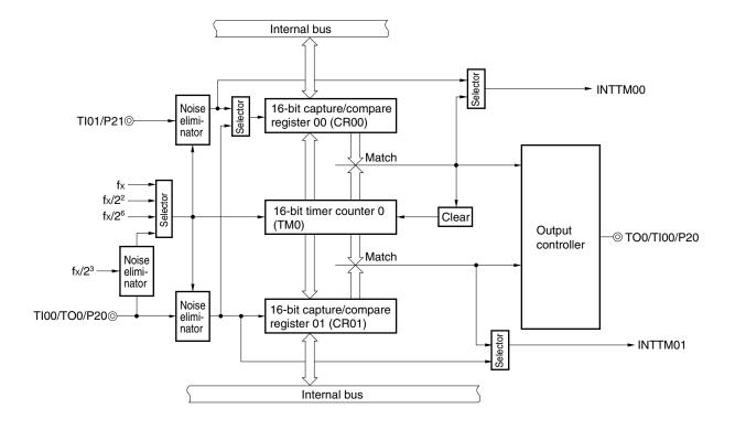
Figure 5-2. Block Diagram of 16-bit Timer/Event Counter 0
