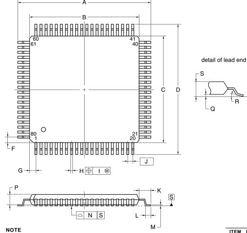
Each lead centerline is located within 0.13 mm of its true position (T.P.) at maximum material condition.
