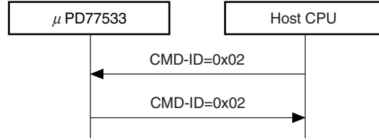
Figure 16-2. FCC Reference Frequency Flow
