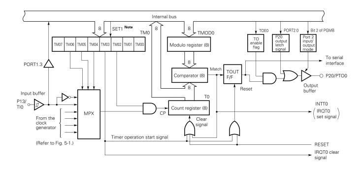
Figure 5-5. Block Diagram of Timer / Event Counter
