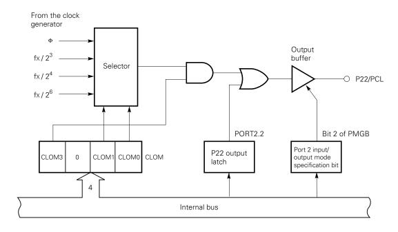
**Remark** Measures are taken to prevent outputting a narrow pulse when selecting clock output enable/disable.
