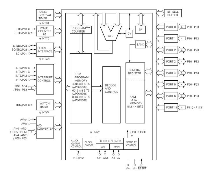
**Note** The  $\mu$ PD75064 uses the program counter of a 12-bit configuration, the  $\mu$ PD75066 and  $\mu$ PD75068 use that of a 13-bit configuration.
