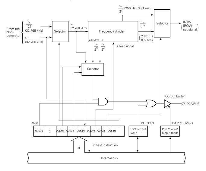
**Remark** () is for fx = 4.194304 MHz, fxT = 32.768 kHz.
