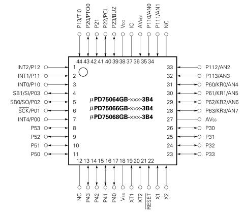
IC : Internally Connected (This pin should be directly connected to VDD)
