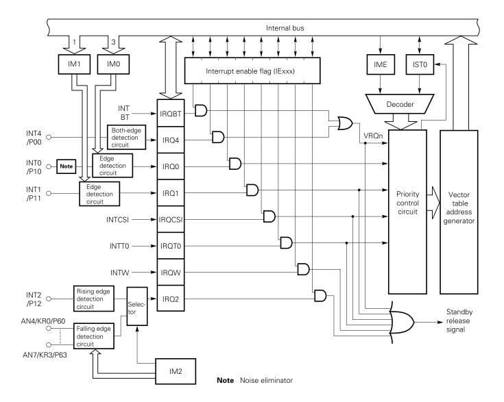
Figure 6-1. Block Diagram of Interrupt Control Circuit
