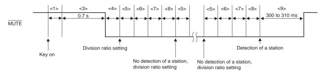
Time <9> is 600 to 610 ms in the case of a band edge.
