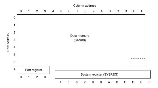
Figure 7-1. Location of System Register on Data Memory
