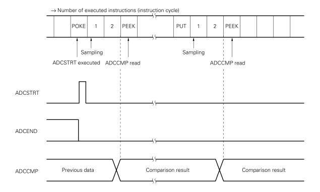
After 1 has been written to ADCSTRT in the single mode (execution of the POKE instruction), a value is stored to ADCCMP three instructions after, and the result of comparison can be read by the PEEK instruction. Even if data is set to ADCR (execution of the PUT instruction), comparison is started in the same manner as ADCSTRT, and the result of comparison can be read three instructions after.
