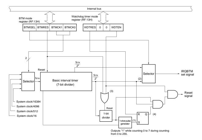
Figure 13-1. Configuration of Basic Interval Timer
