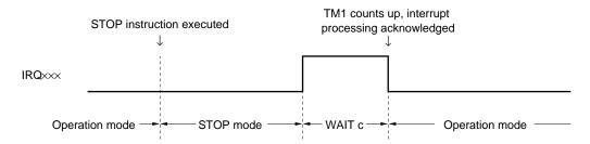
WAIT c : Wait time until TM1 counts clocks divided by m n times  $n \times m/f \\ x + \alpha \ (n \ and \ m \ are \ values \ immediately \ before \ STOP \ mode \ is \ set)$   $\alpha$  : Oscillation growth time (differs depending on the oscillator)
