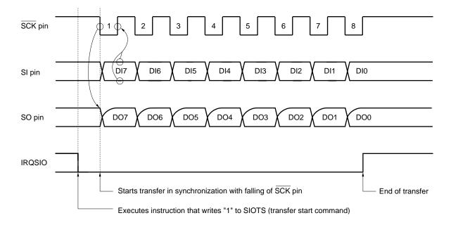
Remark DI: serial data input DO: serial data output
