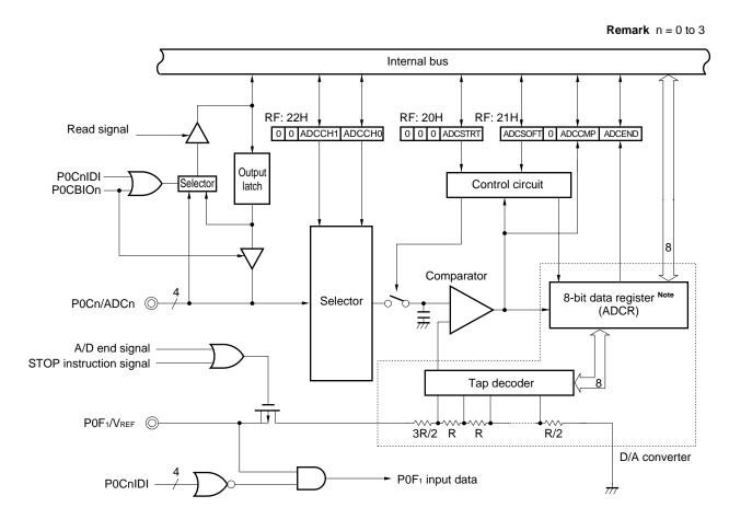
Note The 8-bit data register (ADCR) is cleared to 00H when the STOP instruction is executed.
