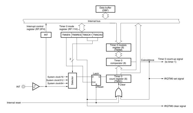
Figure 12-1. Configuration of 8-Bit Timer/Counter
