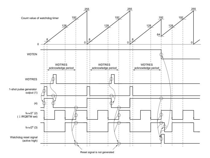
Figure 13-4. Timing Chart of Watchdog Timer (when WDTRES flag is used)
