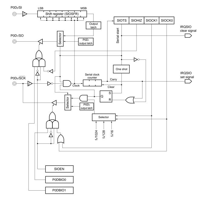
Figure 15-1. Block Diagram of Serial Interface
