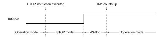
WAIT c : Wait time until TM1 counts clocks divided by m n times  $n\times m/f_X + \ \alpha \ (n \ and \ m \ are \ values \ immediately \ before \ STOP \ mode \ is \ set)$   $\alpha$ : Oscillation growth time (differs depending on the oscillator)
