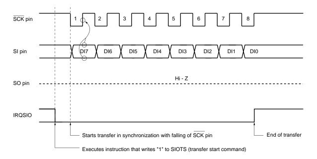
Figure 15-3. Timing in 8-Bit Reception Mode
