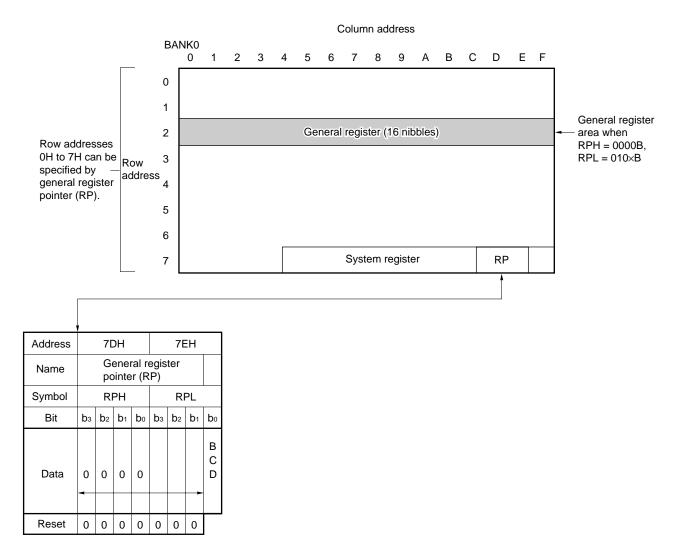
Figure 6-1. Configuration of General Register Pointer
