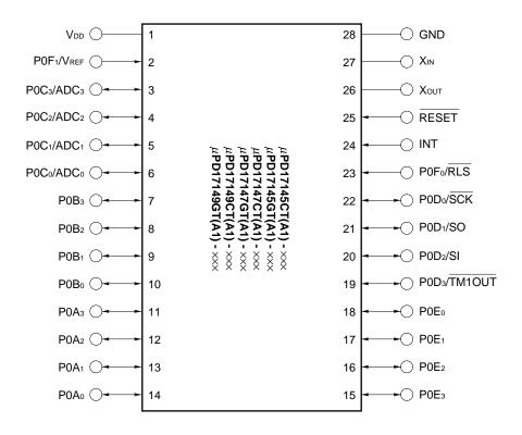
ADC<sub>0</sub>-ADC<sub>3</sub> : analog input GND : ground
