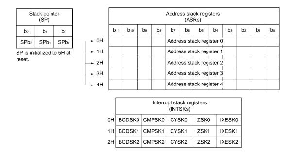
Figure 4-1. Configuration of Stack
