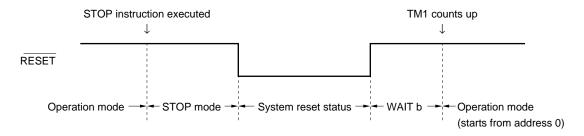
WAIT b : Wait time until TM1 counts 256 clocks divided by 128  $256 \times 128 / \text{fx} + \alpha \text{ (apporox. 4 ms + } \alpha \text{ at fx} = 8 \text{ MHz})$   $\alpha$  : Oscillation growth time (differs depending on the oscillator)
