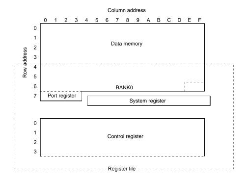
Figure 8-2. Relationships between Register File and Data Memory
