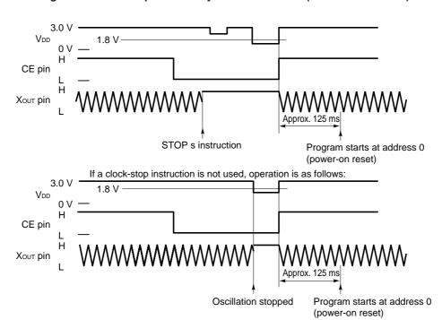
Fig. 14-4 Clock-Stop Release by Power-On Reset ( $T_A = -10$  to +50 °C)
