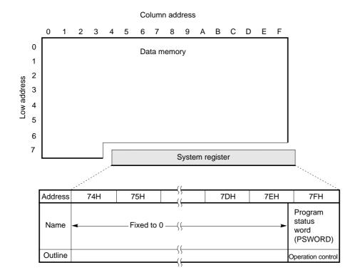
Fig. 5-1 Location on Data Memory and Outline of System Registers
