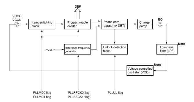
Fig. 11-1 PLL Frequency Synthesizer
