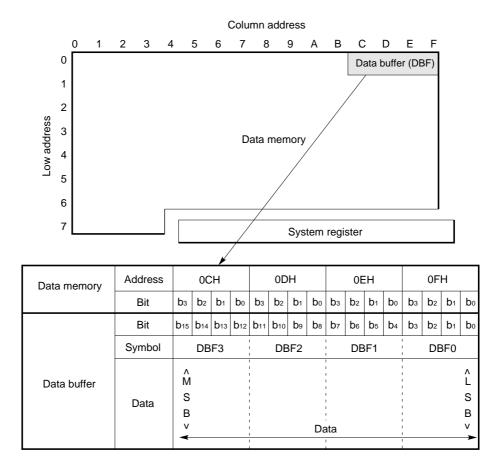
Fig. 8-2 Configuration of the Data Buffer
