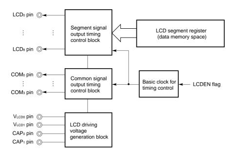
Fig. 13-1 Overview of LCD Controller/Driver
