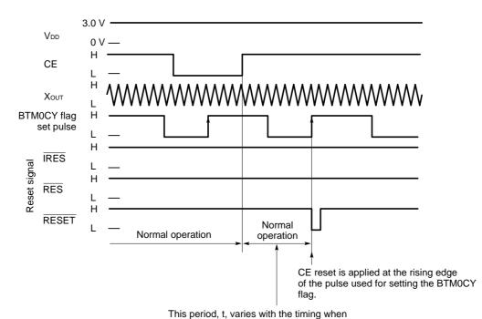
Fig. 15-4 CE Reset Operation When Clock-Stop Not Used
