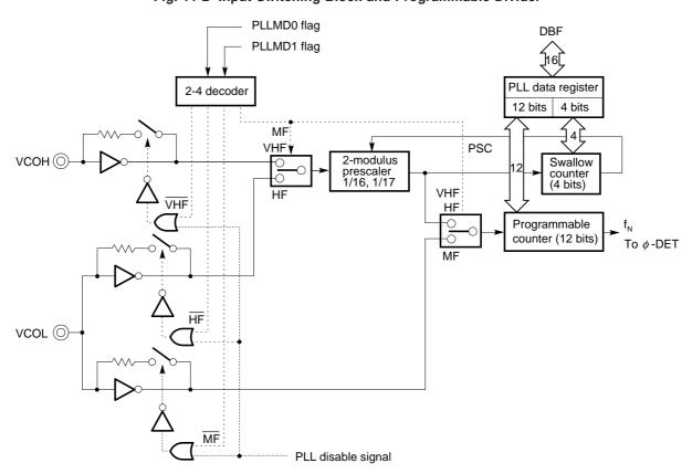
Fig. 11-2 Input Switching Block and Programmable Divider
