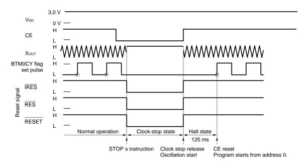
Fig. 15-5 CE Reset Operation When Clock-Stop Used
