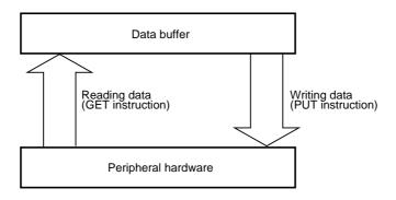
Fig. 8-2 shows the configuration of the data buffer.
