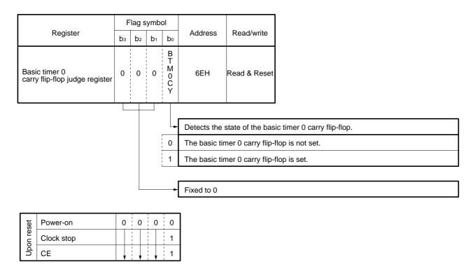
Fig. 10-3 Configuration of the Basic Timer 1 Carry Flip-Flop Judge Register
