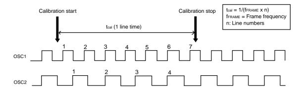
Figure 5–14. Calibration Function Timing (LTS [R1] = 0)
