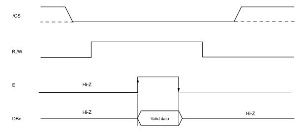
Figure 5-4. M68 Series Interface Data Bus Status (when data read)
