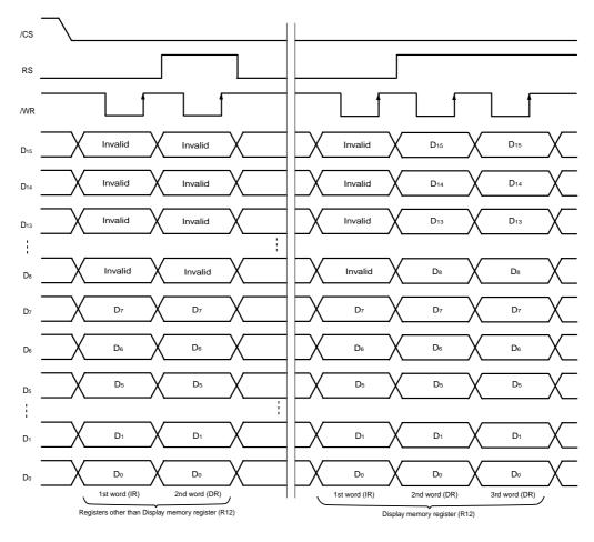
Figure 5–1. Example of 16-bit Data Access (i80 series interface, BMD = 0)
