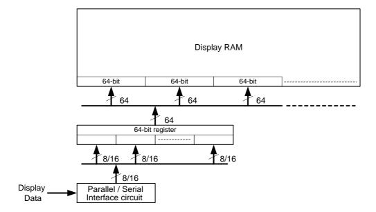
Figure 5-11. Image of Operation in High-speed Write Mode
