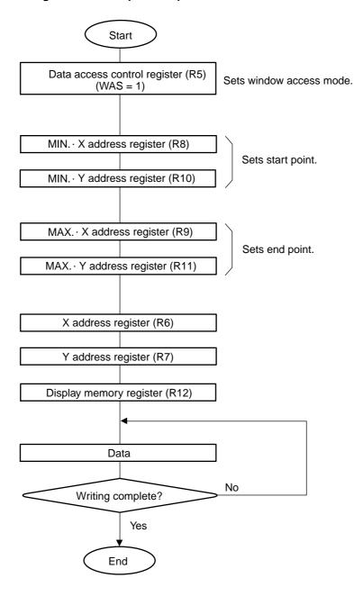
Figure 5–10. Example of Sequence in Window Access Mode
