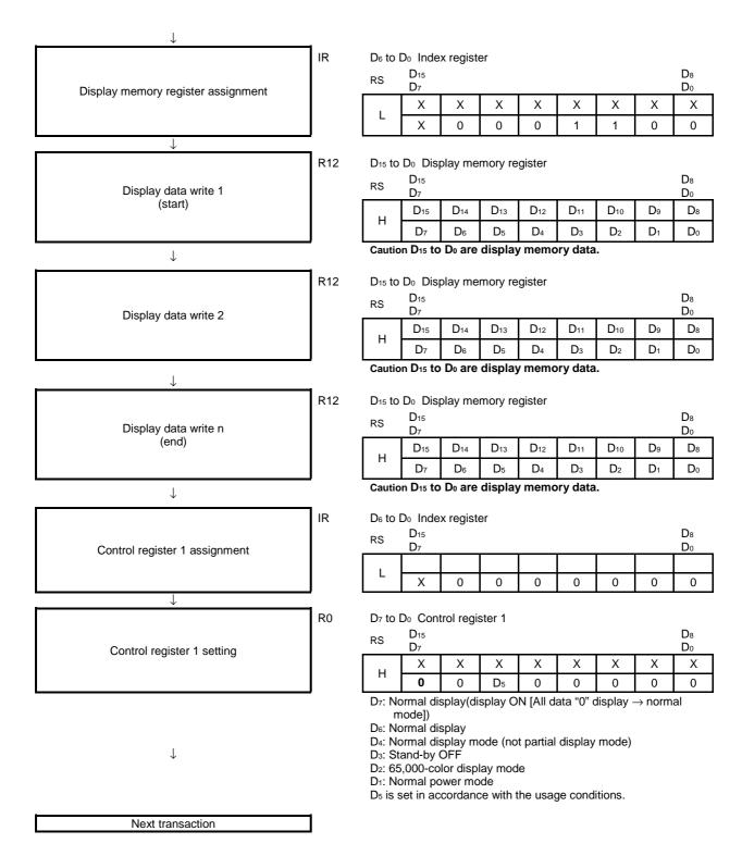
Caution This sequence is shown only for the purpose of illustrating the sequence from power application to display ON, and is not meant for use in mass production design. Note also that this sequence differs depending on the configuration of the chipset and TFT-LCD module
