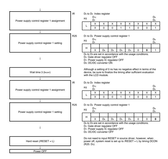
Caution This sequence is shown only for the purpose of illustrating the sequence up to when the power is turned off, and is not meant for use in mass-prodution design. Note also that this sequence differs depending on the configuration of the chipset and TFT-LCD module.
