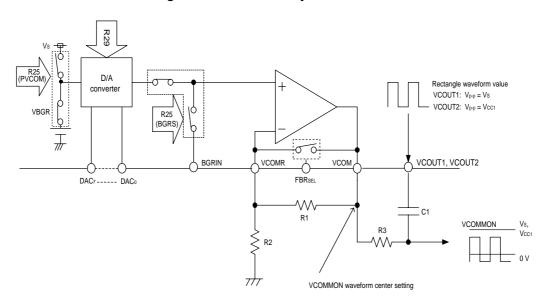
Figure 5-21. Common Adjustment Circuit
