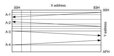
Figure 5–7. Combination of INC, XDIR, and YDIR, and Address Scanning Image
