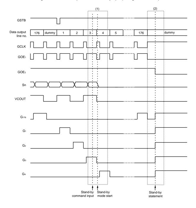
Figure 5–17. Normal Operation → Stand-by Input (during line inversion)
