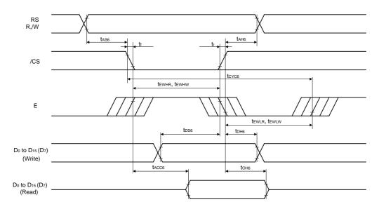
When Vcc1 = 2.5 to 3.6 V, Vcc2 = 2.5 to 3.6 V, Vcc1 ≥ Vcc2 (normal mode, R114 and R115 = 03H)
