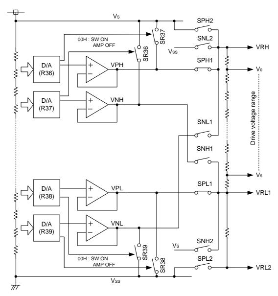
Table 5–14.  $\gamma$ Curve Correction Circuit ( $\gamma$ correction resistance)
