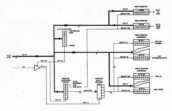
Figure 3. UM83C001 Register Addresses and Selection
