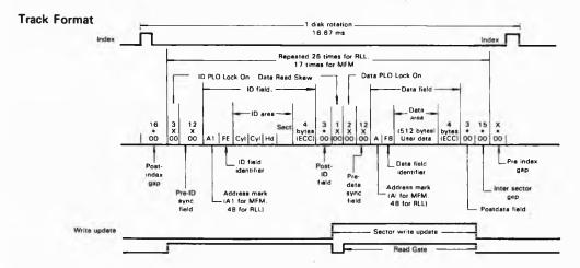
Figure 1, UM83C001 Track Format Diagram
