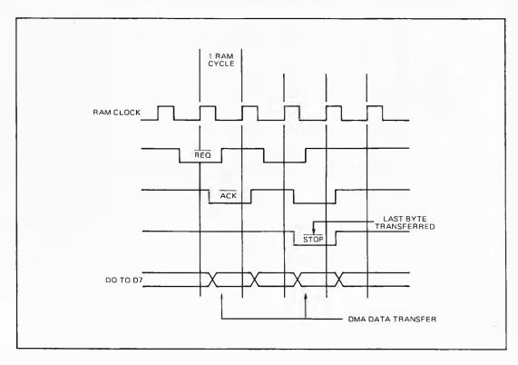
Figure 4. DMA Data Transfer Cycles
