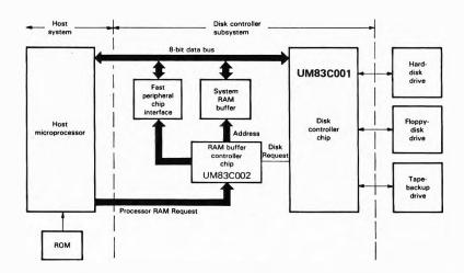
Figure 2. 8086/8088 System with UM83C001 and UM83C002
