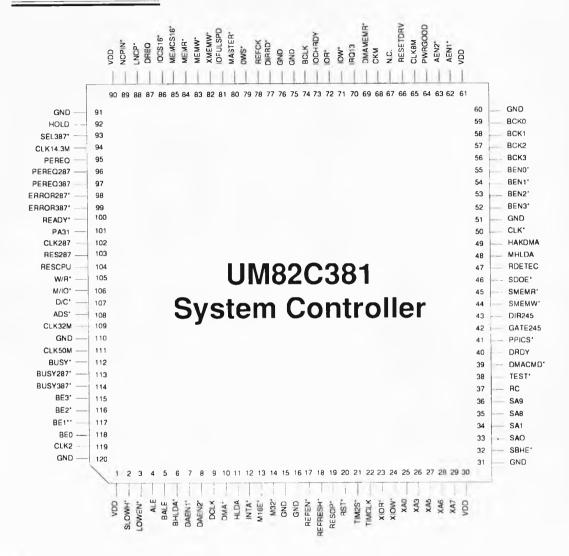
Figure 2. Pin Configuration
