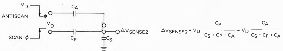
Figure 3b. Equivalent circuit for Capacitive Key with Antiscan Consideration
