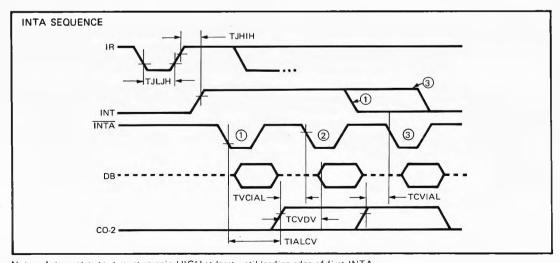
Notes: Interrupt output must remain HIGH at least until leading edge of first INTA.
