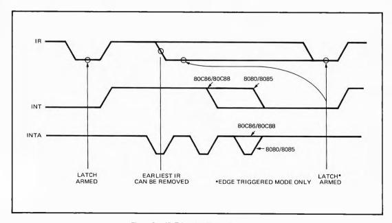
Figure 8. IR Triggering Timing Requirements
