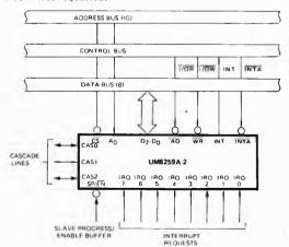
Figure 3. UM8259A-2 Interface to Standard System Bus
