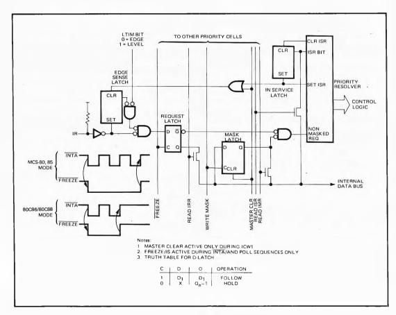
Figure 7. Priority Cell-Simplified Logic Diagram
