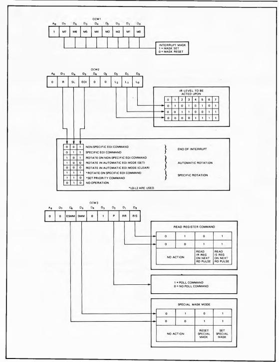
Figure 6. Operation Command Word Format
