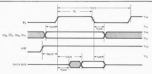
Figure 3. "Read" Timing Characteristics
