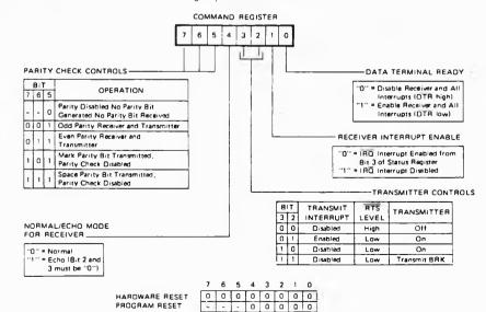
Figure 7. Command Register Format
