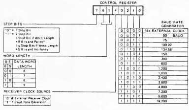
\* This allows for 9-bit transmission (8 data bits plus parity)
