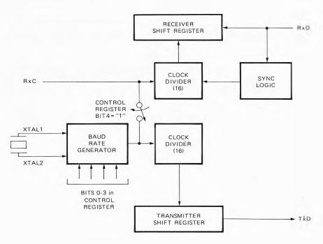
Figure 5. Transmitter/Receiver Clock Circuits
