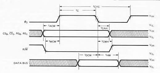
Figure 2. "Write" Timing Characteristics
