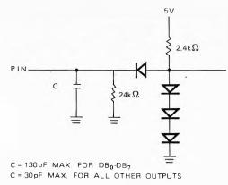
OPEN COLLECTOR OUTPUT TEST LOAD
