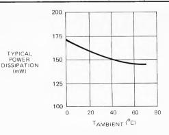
Figure 1. Power Dissipation vs. Temperature
