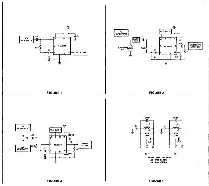
NOTES: 1. Phase shift network is specified in Figure 4. 2. All capacitors in microfarads unless otherwise noted.
