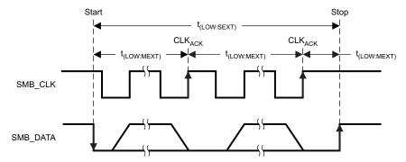
Figure 1. I<sup>2</sup>C/SMBus/PMBus Timing in Extended Mode Diagram
