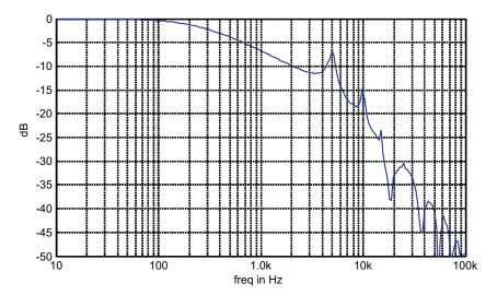
Figure 11. Averaging Filter for Current Monitoring
