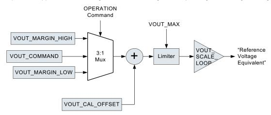
Figure 6. PMBus Voltage Adjustment Methods
