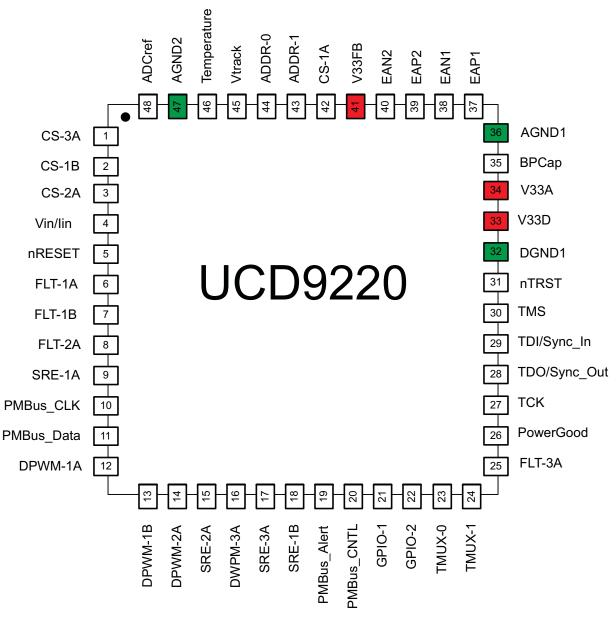
Figure 2. UCD9220 Pin Assignment
