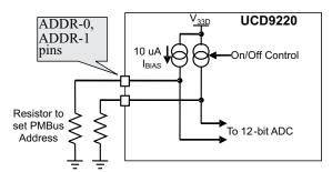
Figure 4. PMBus Address Detection Method
