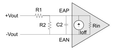
Figure 8. Input Offset Equivalent Circuit
