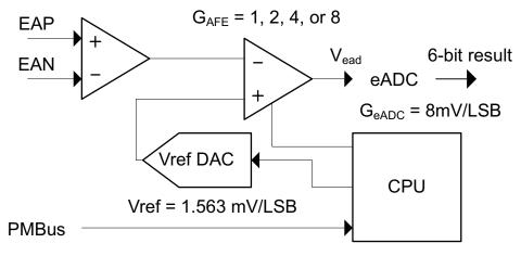
Figure 7. Analog Front End Block Diagram
