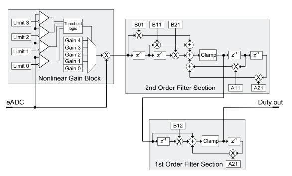
Figure 9. Digital Compensator
