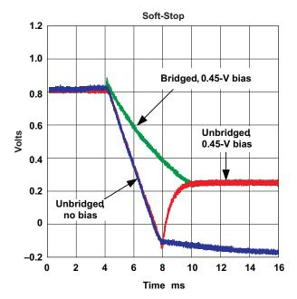
Figure 12. Start and Stop Ramps
