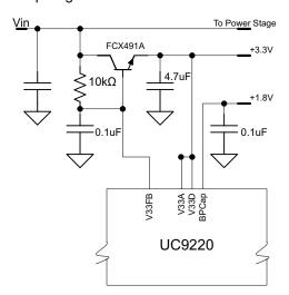
Figure 5. 3.3V Regulator Circuit
