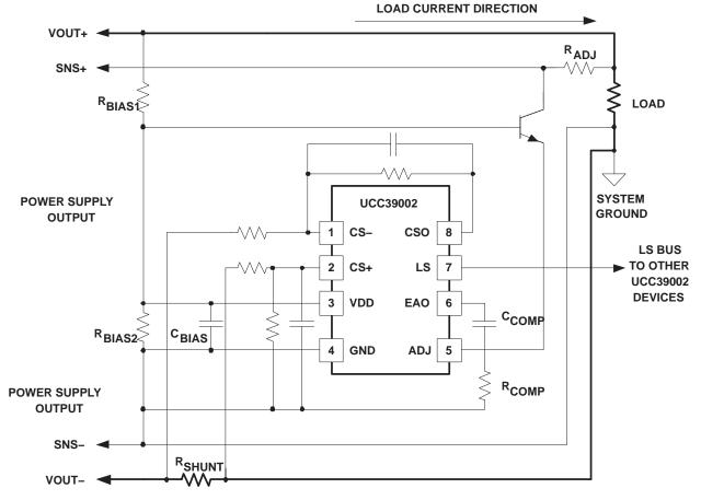
The CSA inputs must be adjusted so as to not exceed their absolute maximum voltage ratings.
