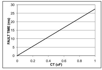
Figure 5. Fault time vs. timing capacitance.
