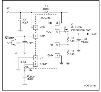
Figure 1. Typical application 5V to 3.3V, 5A
