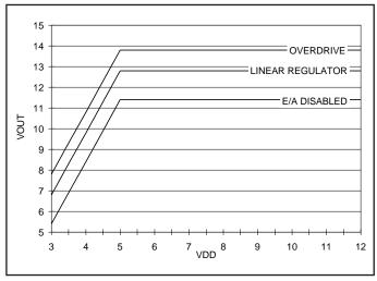
Figure 2. Typical V<sub>OUT(max)</sub> vs. VDD.
