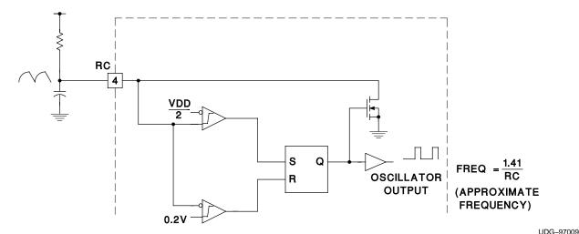
NOTE: The oscillator generates a sawtooth waveform on RC. During the RC rise time, the output stages alternate on time, but both stages are off during the RC fall time. The output stages switch a ½ the oscillator frequency, with guaranteed duty cycle of < 50% for both outputs.
