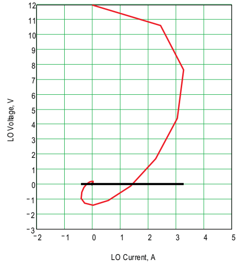
Figure 25. Turn-Off Voltage and Current Switching Diagram
