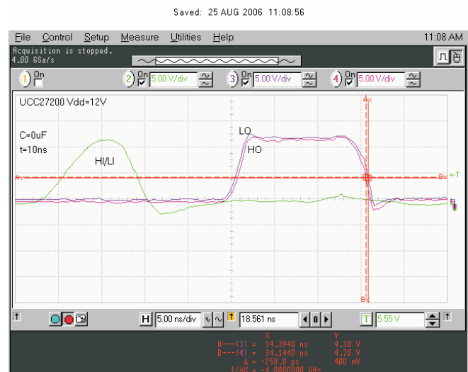
Figure 34. 10-ns Input Pulse Delay Matching
