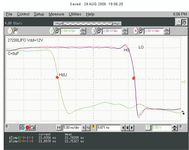
Figure 32. V_{LO} and V_{HO} Falling Edge Delay Matching
