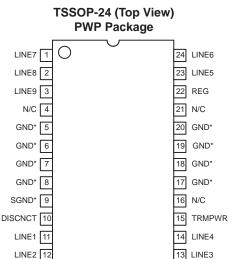
\* PWP package pin 9 serves as signal ground; pins 5, 6, 7, 8, 17, 18, 19 and 20 serve as heatsink/ground.
