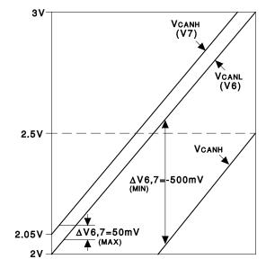
NOTE: Valid output of CANH, CANL during recessive state transmission. TXD = LOGIC 1
