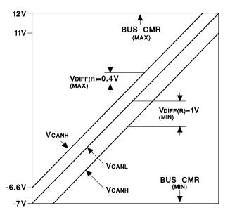
NOTE: Valid voltage range of V<sub>CANH</sub> for sensing dominant bus state as V<sub>CANL</sub> varies over bus common range mode. TXD = LOGIC1 UDG-96205
