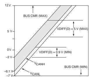
NOTE: Valid voltage range of V<sub>CANH</sub> for sensing dominant bus state as V<sub>CANL</sub> varies over bus common mode range. TXD = LOGIC 0 UDG-97160
