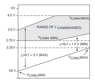
NOTE: Valid voltage range of V<sub>CANH</sub> for sensing dominant bus state as V<sub>CANL</sub> varies. TXD = LOGIC 0
