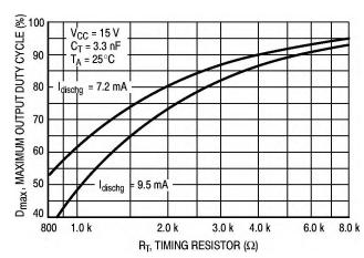
Figure 5. Maximum Output Duty Cycle versus Timing Resistor
