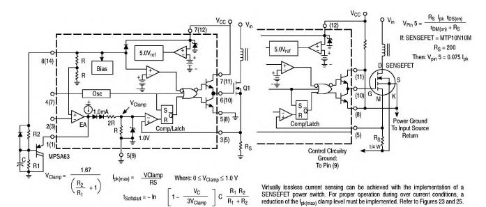
Figure 25. Adjustable Buffered Reduction of Clamp Level with Soft-Start
