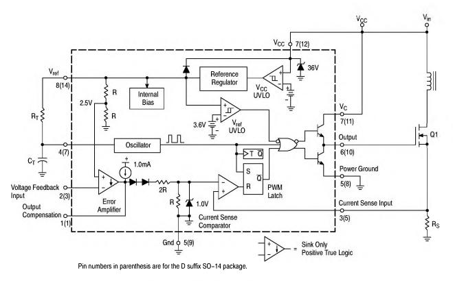
Figure 18. Representative Block Diagram
