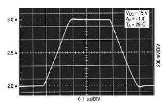
Figure 7. Error Amp Large Signal Transient Response
