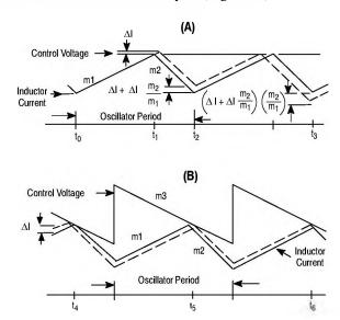
Figure 20. Continuous Current Waveforms
