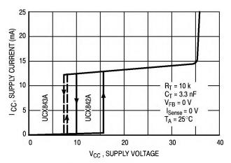
Figure 17. Supply Current versus Supply Voltage
