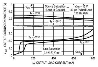
Figure 14. Output Saturation Voltage versus Load Current
