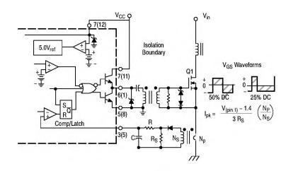
Figure 30. Isolated MOSFET Drive
