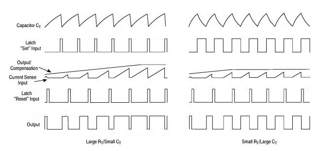
Figure 19. Timing Diagram
