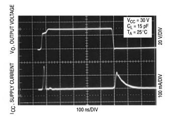
Figure 16. Output Cross Conduction
