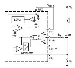
Series gate resistor  $R_g$  will damp any high frequency parasitic oscillations caused by the MOSFET input capacitance and any series wiring inductance in the gate–source circuit.
