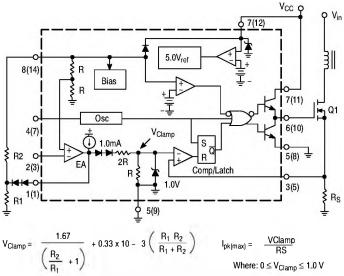
Figure 23. Adjustable Reduction of Clamp Level
