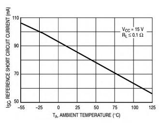
Figure 11. Reference Short Circuit Current versus Temperature
