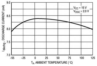
Figure 4. Oscillator Discharge Current versus Temperature
