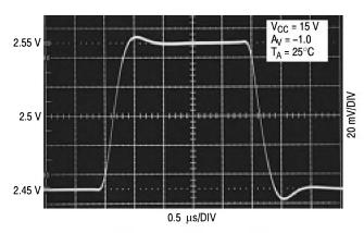
Figure 6. Error Amp Small Signal Transient Response
