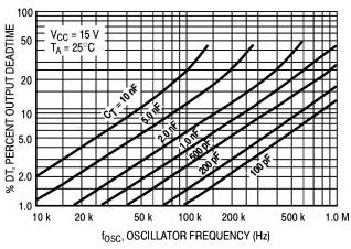
Figure 3. Output Deadtime versus Oscillator Frequency
