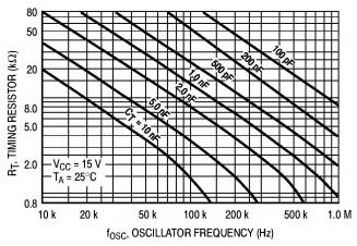
Figure 2. Timing Resistor versus Oscillator Frequency
