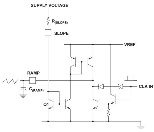
Figure 11. Voltage Mode Operation
