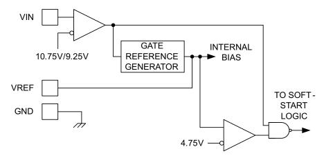
Figure 3. Undervoltage Circuit
