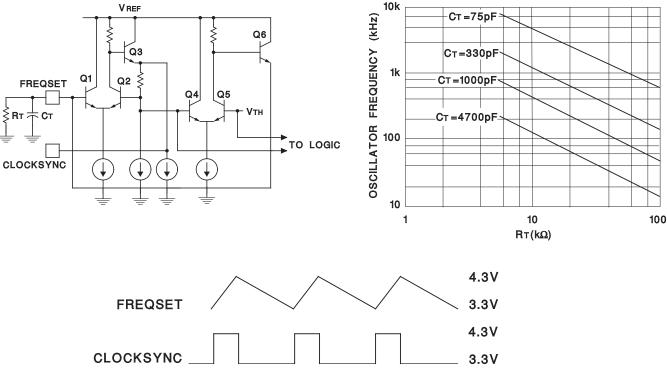
Figure 4. Simplified Oscillator Schematic
