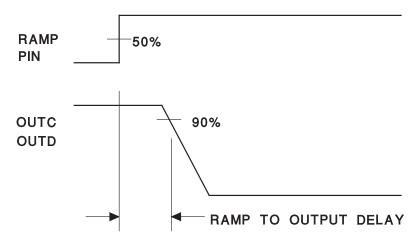
Figure 2. Ramp to Delay Output
