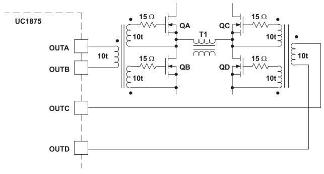
Figure 8. 3 Winding Bifilar, AWG 30 Kynar Insulation
