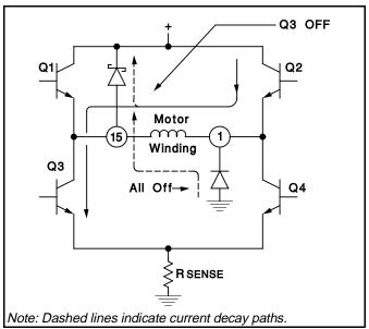
Figure 7: Simplified Schematic of Output Stage
