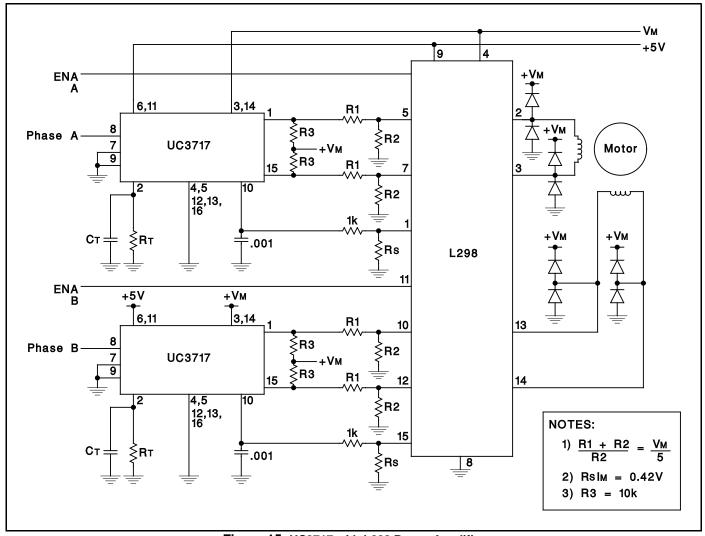
Figure 15: UC3717 with L298 Power Amplifier
