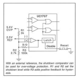
Figure 7. Over-Voltage Protection
