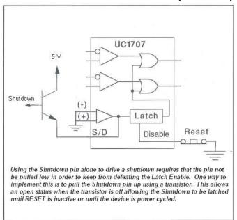
Figure 4. Use of the Shutdown Pin
