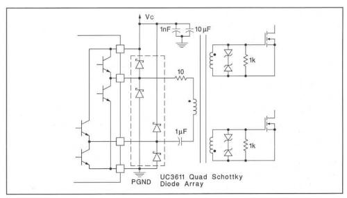
Figure 5. Transformer Coupled Push-Pull MOSFET Drive Circuit
