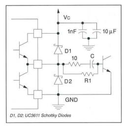
Figure 10. Power Bipolar Drive Circuit
