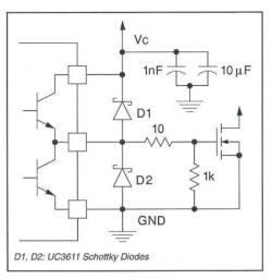
Figure 8. Power MOSFET Drive Circuit
