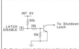
The Shutdown latch is disabled when pin 3 is open. An impedance of 4k or less from pin 3 to ground will allow a shutdown signal to set the latch which can then be reset by either recycling the VIN supply or by momentarily (>200ns) raising pin 3 high.
