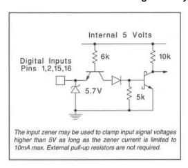
Figure 2. Typical Digital Input Gate
