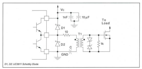
Figure 11. Transformer Coupled MOSFET Drive Circuit
