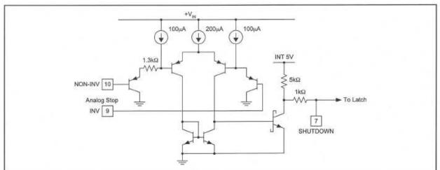
The input common-mode voltage range is from ground to (VIN-3V). When not used both inputs should be grounded. Activate time is a function of overdrive with a typical value of 180ns. Pin 7 serves both as a comparator output and as a common digital shutdown input. A high signal here will accomplish the fastest turn off of both outputs. Note that "OFF" is defined as the outputs low. Pulling shutdown low defeats the latch operation regardless of its status.
