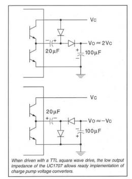
Figure 9. Charge Pump Circuits
