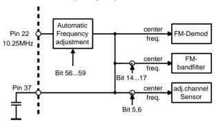
For fine tuning, the center frequency of all these integrated active filters (band filter, demodulator and adjacent channel sensor) can be shifted in steps of 6.25 kHz by means of Bit 56 to Bit 59. Additionally, the center frequency of the band filter can be adjusted separately by means of Bit 14 to Bit 17 if Bit 4 is set to 1. If Bit 4 is set to 0, the default setting is used.
