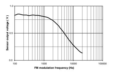
Figure 17. FM Input Level Sweep
