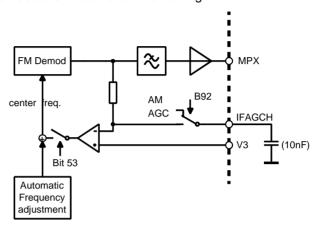
The center frequency of the FM demodulator can be adjusted by means of Bit 56 to 59. At the center frequency, the DC voltage at the MPX output Pin 11 is equal to the MPX offset voltage that can be measured at Pin 11 while MPX mute is active (Bit 7 = 1). This adjustment will affect the center frequency of all integrated filters as mentioned before.
