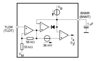
Figure 14. Generation of Control Voltage (CT) for Mode Switching
