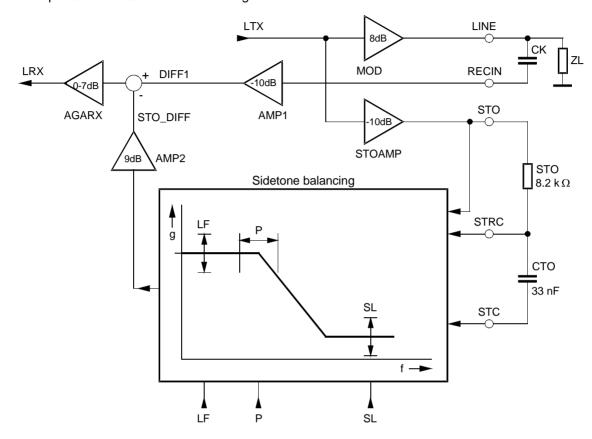
The Side Tone Balancing (STB) has the task of reducing the cross-talk from LTX (microphone) to LRX (earpiece) in the frequency range of 0.3 to 3.4 kHz. The LTX signal is converted into a current in the MOD block. This current is transformed into a voltage signal (LINE) by the line impedance ZL. The LINE signal is fed into the summing amplifier DIFF1 via capacitor CK and attenuator AMP1.
