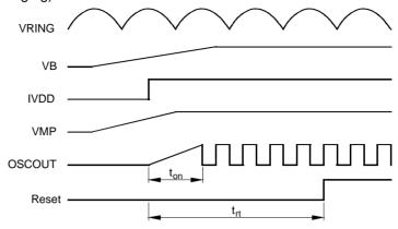
Figure 11. Power-on Reset (Low Voltage Reset)
