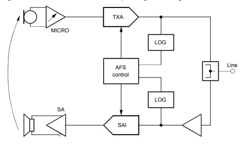
Figure 16. Block Diagram Hands-free Mode U4091BM-N 4-point Signal Sensing
