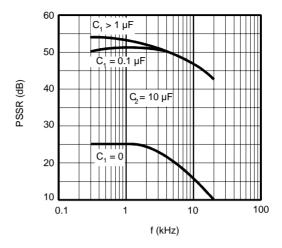
**Figure 7.** Power Supply Rejection versus Frequency —  $C_2 = 5 \mu F$
