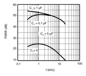
**Figure 8.** Power Supply Rejection versus Frequency —  $C_2$  = 1  $\mu F$
