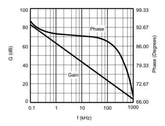
Figure 5. Differential Gain versus Frequency
