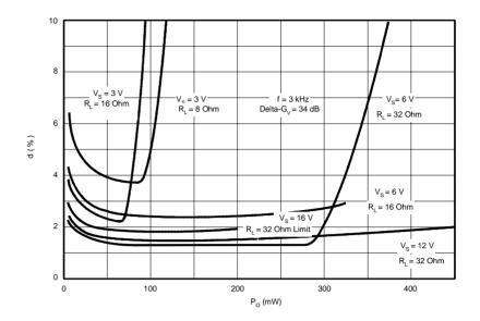
**Figure 15.** Distortion versus Power — f = 1 or 3 kHz, Delta- $G_V = 12$  dB
