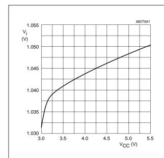
Fig.9 Input voltage as a function of the supply voltage.
