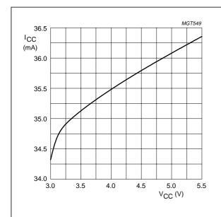
Fig.7 Supply current as a function of the supply voltage.
