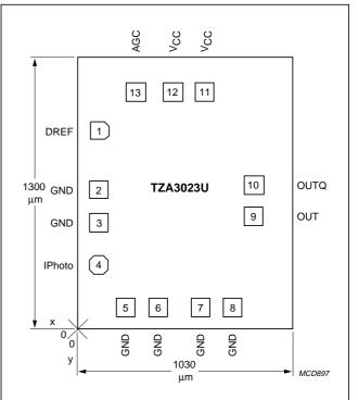
Fig.22 Bonding pad locations of the TZA3023U.
