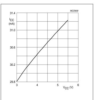
Fig.9 Supply current as a function of the supply voltage.
