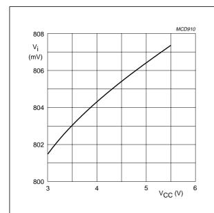
Fig.10 Input voltage as a function of the supply voltage.
