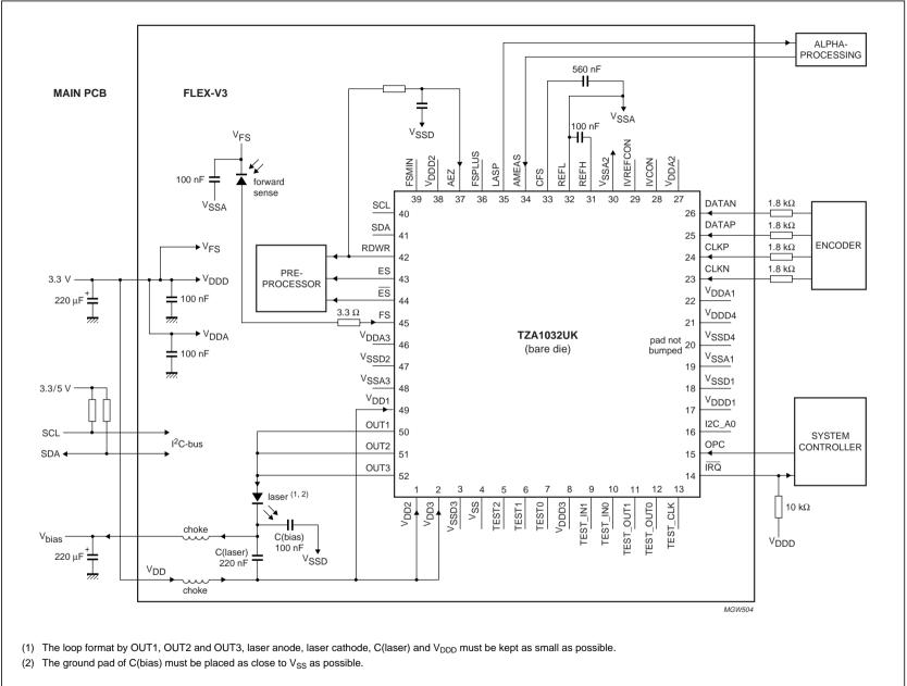
Fig.4 Typical application diagram for TZA1032UK on flex foil.
