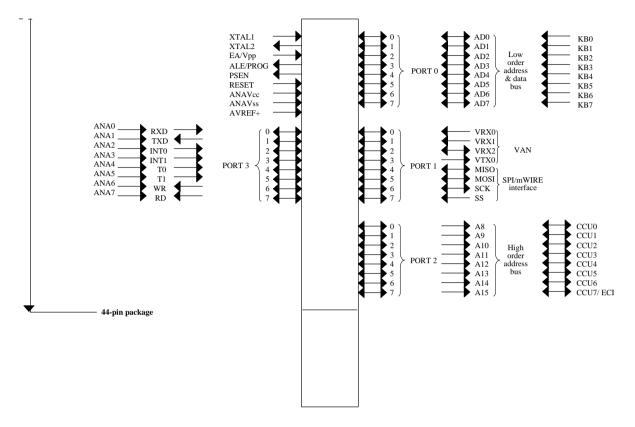
Figure 2. TSC8051A30 pin functions
