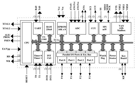
(1): Alternate function of Port 1 (2): Alternate function of Port 2 (3): Alternate function of Port 3 (0): Alternate function of Port 0
