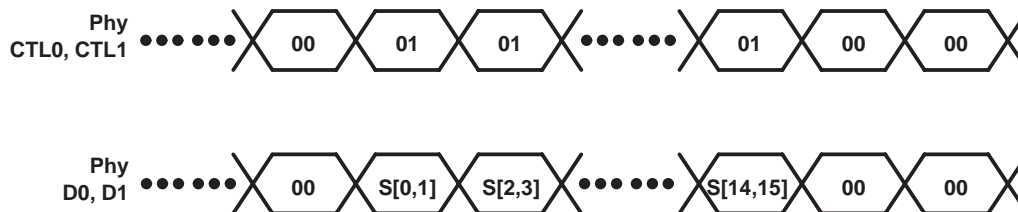
Figure 6. Status Transfer Timing
