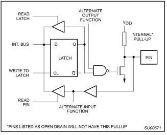
Figure 2. Typical Port Bit Latches and I/O Buffers
