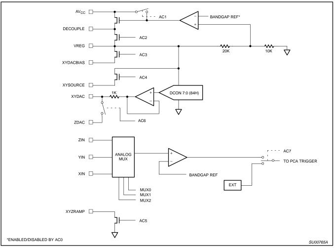
Figure 1. Analog Section
