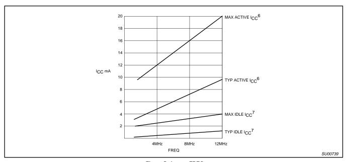
Figure 5.  $I_{CC}$  vs. FREQ Maximum  $I_{CC}$  values taken at  $V_{CC}$  = 5.5V and worst case temperature. Typical  $I_{CC}$  values taken at  $V_{CC}$  = 5.0V and 25°C. Notes 6 and 7 refer to AC Electrical Characteristics.
